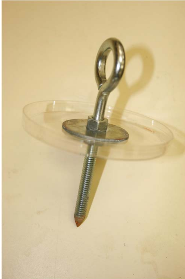
Fig. 1 Bait station constructed to hold liquid protein and carbohydrate solutions. Stations were designed to be secured into a soil substrate.
