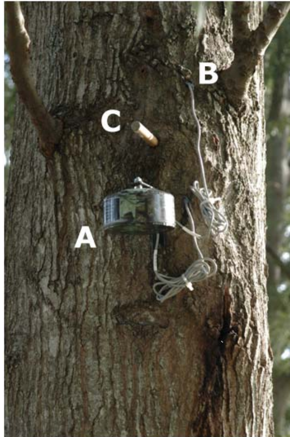
Fig. 2. Weatherproof station (A) on a tree with thermocouples (B) inserted in Camponotus pennsylvanicus (DeGeer) nest galleries. Wooden dowel (C) inserted into tree hole was used for accessing galleries to verify nest activity with a borescope.
